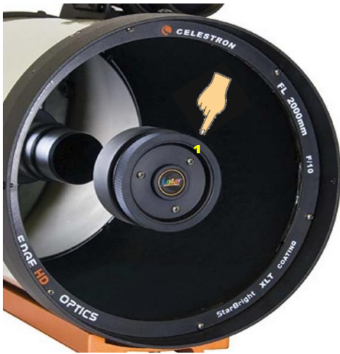
Shadow of a finger next to the collimation screw (of M2) labeled #1
