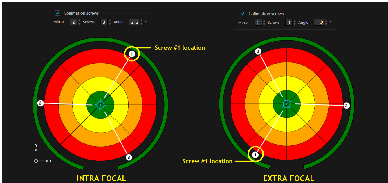
Collimation screw location in SKW CT for INTRA versus EXTRA focal images
