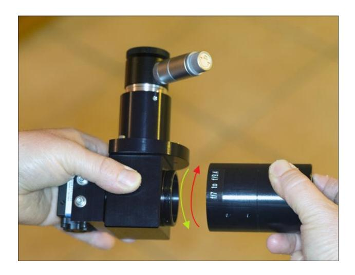
Then screw the module you plan to use for the given F/ ratio from the system to measure.
