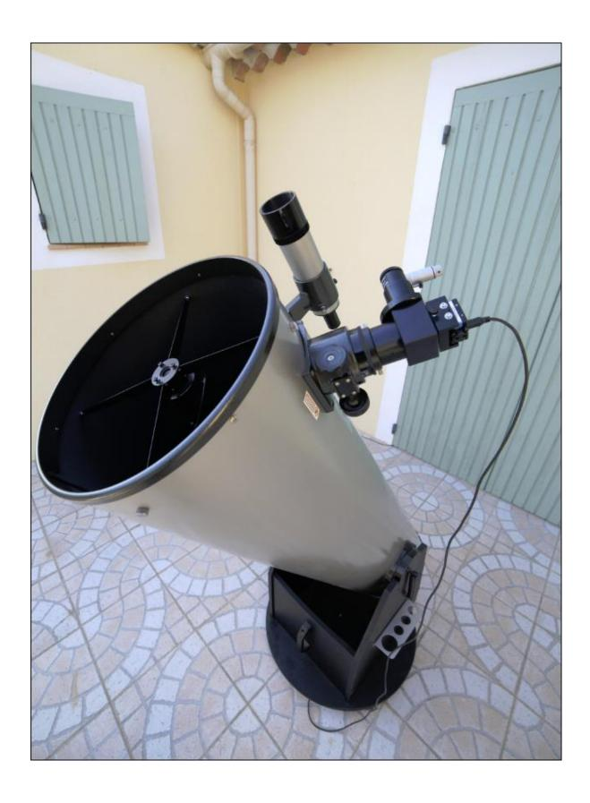
The star shall be centered with the eyepiece the same way it was with the calibration pinhole. As well as the focus shall be adjusted the same way.
