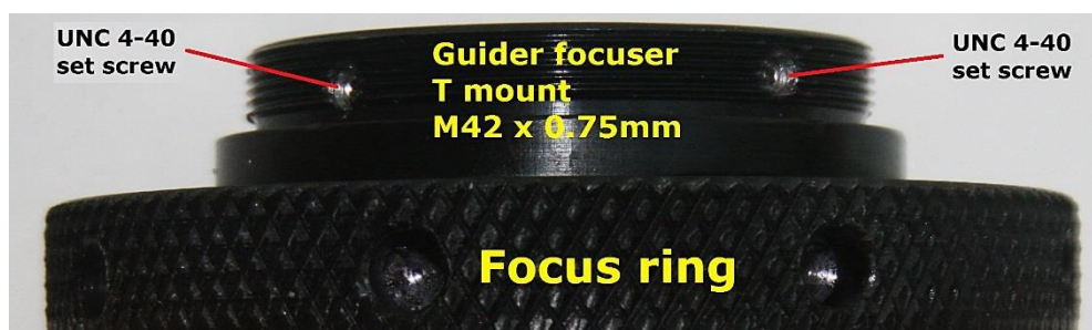
ONAG guider helical focuser and its set screws
